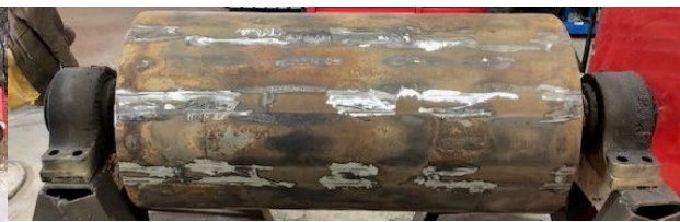
Rebuilding Head pulley
