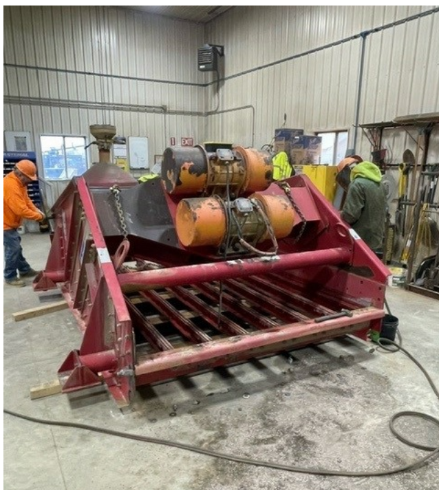
Brian Pies and Lee Wright from Summit rebuilding a dewatering screen.
